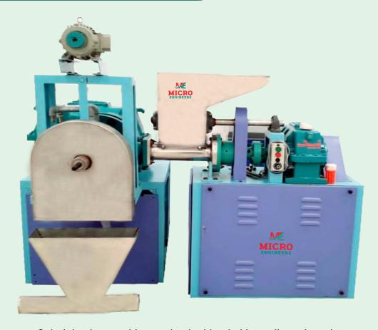
Gelatinization machine cooks the blended ingredients by using pre-set temperature condition of the barrel in such a manner that material be completely and uniformly gelatinized and at the end of this process, it cuts in a small sphere shape.
