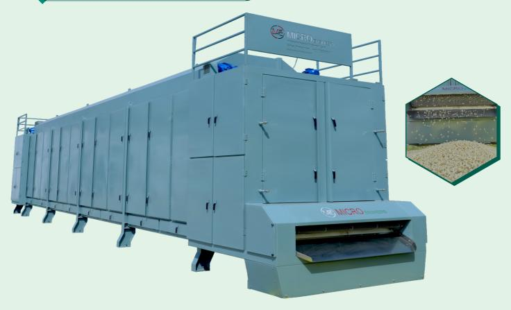
The Continuous Dryer operates by pulling hot hair through the materials and gives the complete dry and ready Fryums which we can directly use for frying process or packing process.
