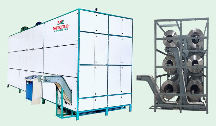
The Continuous Dryer operates by pulling hot hair through the materials and gives the complete dry and ready Fryums which we can directly use for frying process or packing process.
